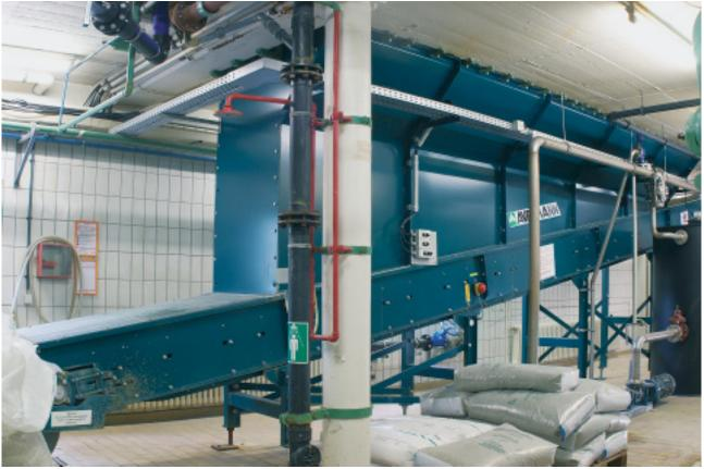
Sliding belt conveyor with special hopper
