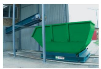
Filter cake conveying machine with shifting platform for an optimum feed of the trough
