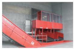
Chain conveyor and sliding belt conveyor
