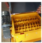
Two-shaft rotors efficiently granulate the material.
