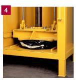
1 Compress your empty drums. 2 Stack and store the compressed drums. 3 The machine is suitable for oil drums and other drums without explosive contents. 4 You are able to reduce the volume of your drums with up to 90%.
