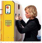
The bale is ejected by a safe two-hand operation.
