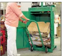
The supplied bale trolley eases bailing and subsequent transport of the bale.
