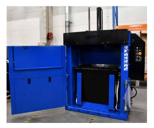
BLUE COLOR RAL 5017 REINFORCED STEEL CONTAINERS / ACTIVATION KEY LOADING DOOR SAFETY LIMIT SWITCH / DISCHARGE DOOR SAFETY LIMIT SWITCH INTELLIGENT SMART TECHNOLOGY EUROPRESS SMART CONNECTIVITY READINESS
