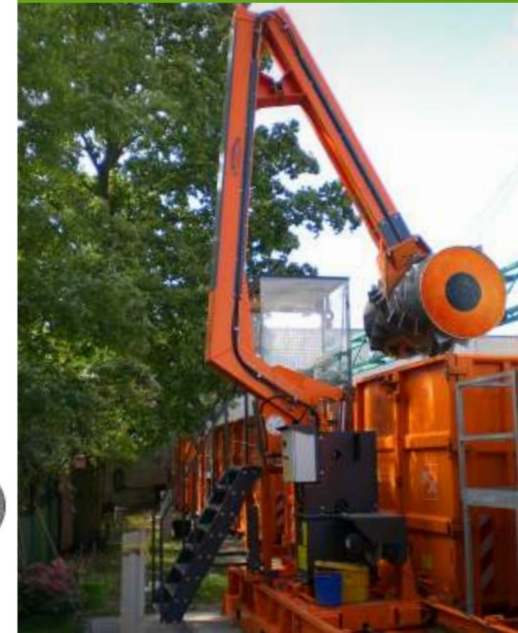
The BERGMANN RPV 7700 Traversing System for several parallel installed containers at one location.
