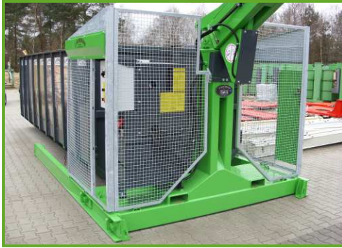
safety grids all around shield the danger zone
