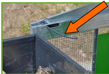
not activated limit switch bar
