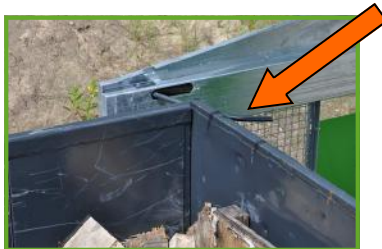
activated limit switch bar
