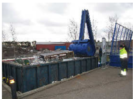
Compaction of metal scrap 2,5:1
