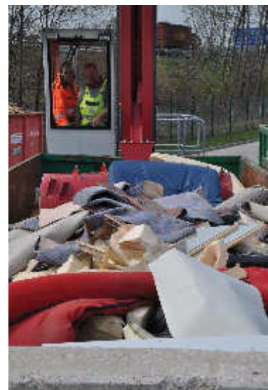
Compaction of bulky waste up to 5:1
