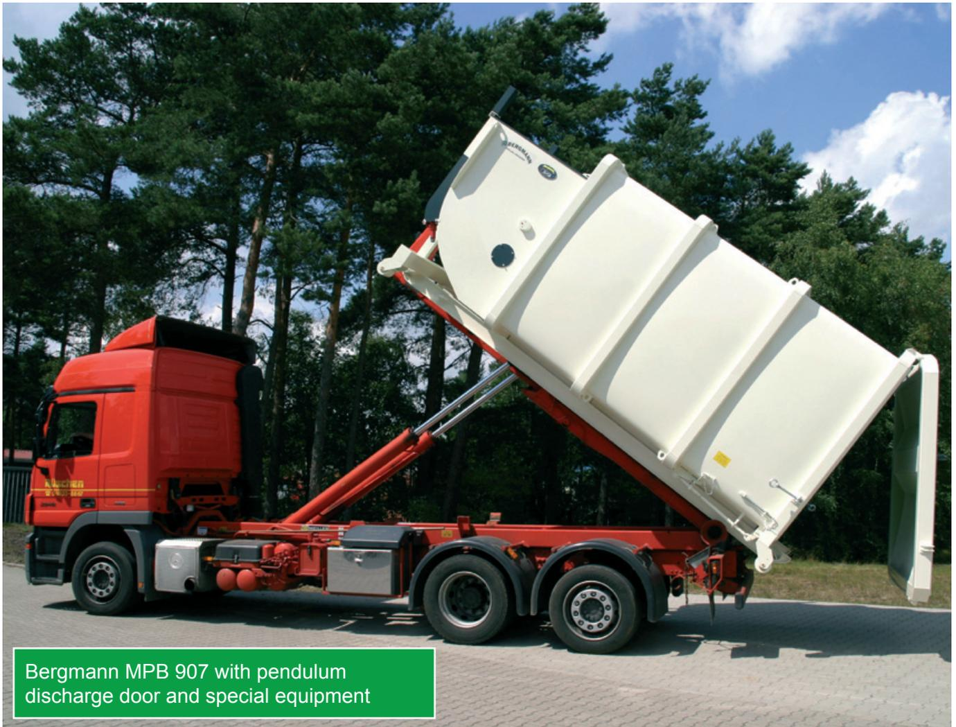
Bergmann MPB 907 with pendulum discharge door and special equipment
