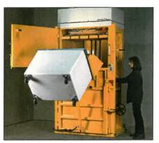
The machine is equipped with a safe twohand operation. The operator is in a safe distance from the lift system, when the lift is in operation.
