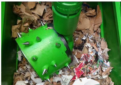
Functioning of the compaction-drum
