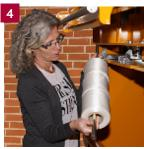
1 Compact your waste and eject the finished bale. 2 Remove and store the bale until collection. 3 With a vertical door opening you have an ergonomical working posture 4 Strap rolls are placed in front, making them easy to replace
