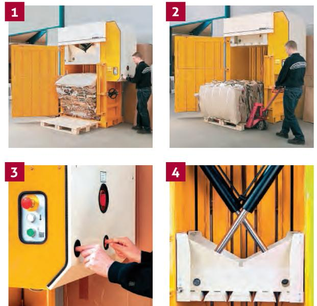
**1** Compact your waste and eject the finished bale. **2** Remove and store the bale until collection. **3** The bale is ejected by a safe two-hand operation. **4** The cross cylinders ensure stable compression and a low overall height.
