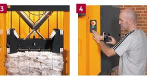
**1** Compact your waste and eject the finished bale. **2** Remove and store the bale until collection. **3** The cross cylinders ensure stable compression and a low overall height. **4** The bale is ejected by a safe two-hand operation.
