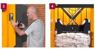
**1** Compact your waste and eject the finished bale. **2** Remove and store the bale until collection. **3** The bale is ejected by a safe two-hand operation. **4** The cross cylinders ensure stable compression and a low overall height.
