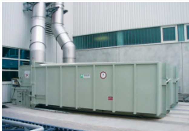
SP12 with transport container and special feeding chute
