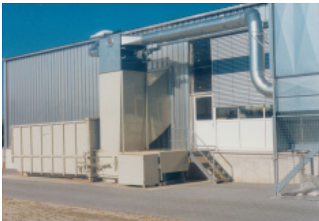
Stationary press with container, hopper and mounted extraction unit
