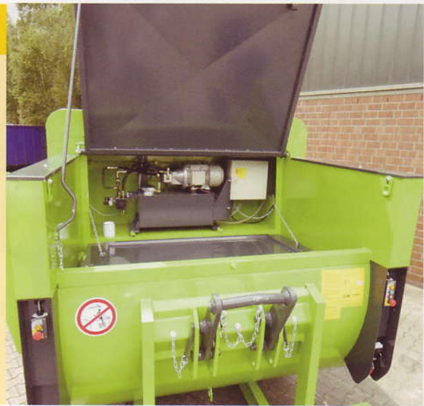
The cover of the aggregate room can be fold down and provides a secure platform for making maintenance work.
