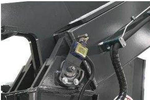
When the drum is lifted completely out of the container the limit switch is activated. Only now it is possible to move the compaction unit laterally to the next container
