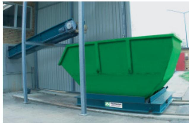
Filter cake conveying machine with shifting platform for an optimum feed of the trough
