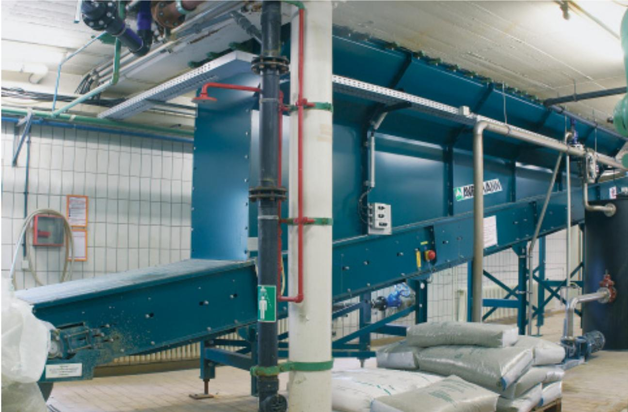
Sliding belt conveyor with special hopper
