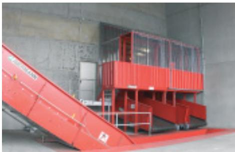
Chain conveyor and sliding belt conveyor
