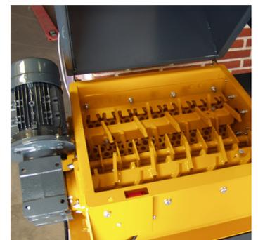
Two-shaft rotors efficiently granulate the material.
