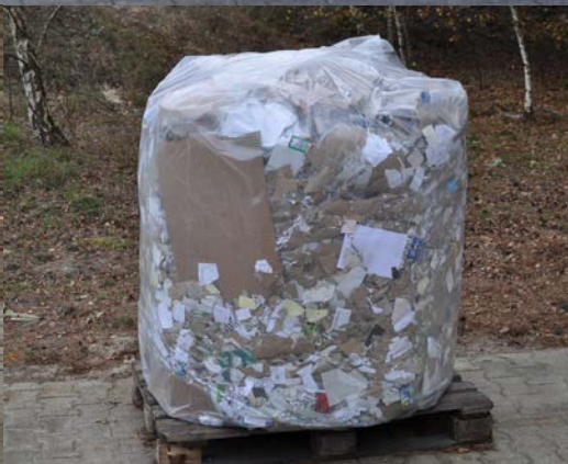
Bale Roto-Compactors PS 8100 & PS 1000-E approx. 300 kg paper and cardboard measurements: L 1.100 x W 1.100 x H 1.100
