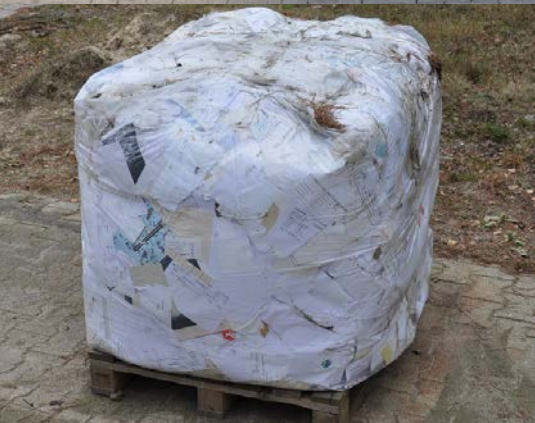
Bale Roto-Compactor PS 1400-E approx. 450 kg paper and cardboard measurements: L 1.200 x W 1.100 x H 1.100
