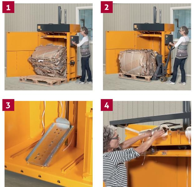
**1** Compact your waste and eject the finished bale. **2** Remove and store the bale until collection. **3** An efficient and silent ejecting system ensures easy handling of the compressed bale. **4** The strap rolls are easy to replace in front of the machine.
