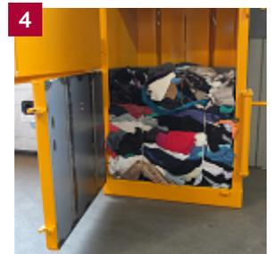
**1** Compact your waste and eject the finished bale. **2** Remove and store the bale until collection. **3** A knife in front of the baler makes it easy to cut the straps to a suitable length. **4** There are no retainers or paint inside the chamber, to prevent damage on the clothes.
