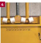
**1** Compact your waste and eject the finished bale. **2** Remove and store the bale until collection. **3** The baler has a simple control panel. **4** Strap rolls are easy to replace in front of the machine.
