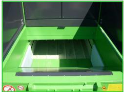
The Alpha Pack bin APB 616 is a mobile press container which can be transported by Roll-On-Off vehicles. The Bergmann working principle compacts cardboard and recyclable fraction in a very efficient unique way.
