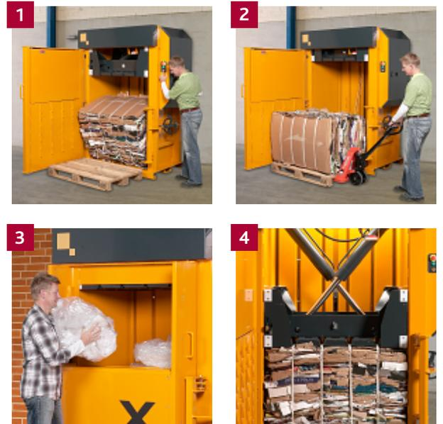
**1** Compact your waste and eject the finished bale. **2** Remove and store the bale until collection. **3** The door to the chamber opens automatically and remains down, giving rational waste filling. **4** The cross cylinders ensure stable compression and a low overall height.
