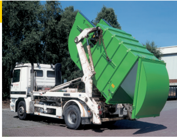
The tapered sides of the container make tipping easy. The unit's pick-up lugs can be adjusted to suit different skiplift vehicles.
