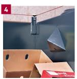
**1** The bale is tied automatically. **2** The finished bales are pushed forward. **3** The baling channel adjusts automatically to keep the bale density constant. **4** The machine is equipped with an automatic light barrier that starts the pressing cycle.
